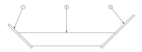
Figure 9.30 51255 Underbody Angled Support Brace
