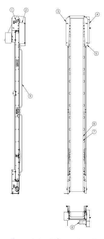
Figure 9.45 51440 12' Conveyor Assembly
