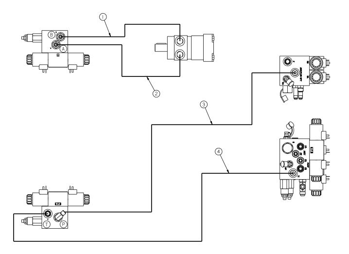
Figure 9.28 26608 Hydraulic Schematic EZ Series II 500 Autoloader
