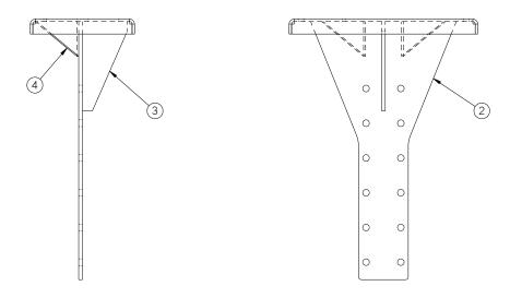
Figure 9.4 51253 Front Leg Support Mounting Plate Assembly
