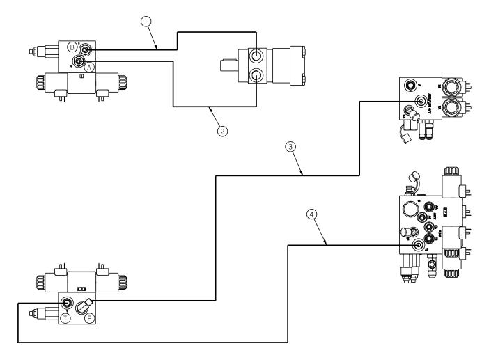
Figure 9.38 26609 Hydraulic Schematic EZ Series II 1000 Autoloader
