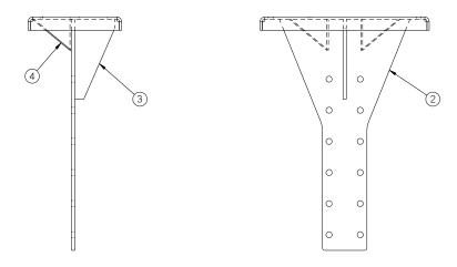
Figure 9.14 51253 Front Leg Support Mounting Plate Assembly
