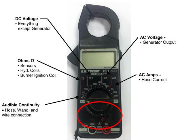
Figure 7.2 Clamp – On Amp Meter/Multimeter
