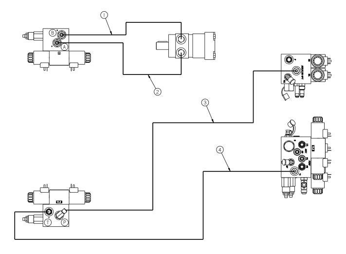
Figure 9.19 26693 Hydraulic Schematic Super Shot Autoloader
