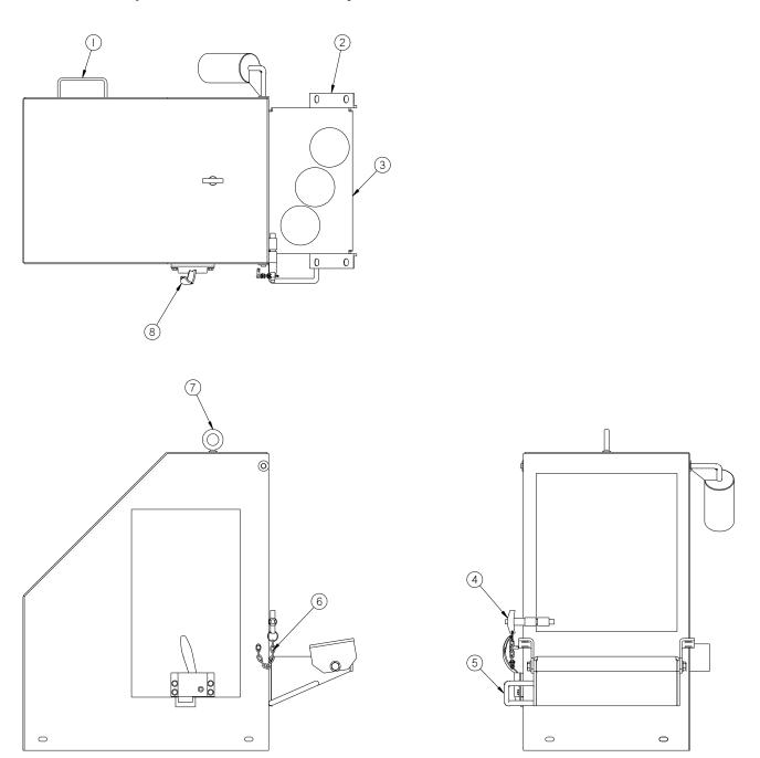
Figure 9.15 51370 Splash Box Welded Assembly
