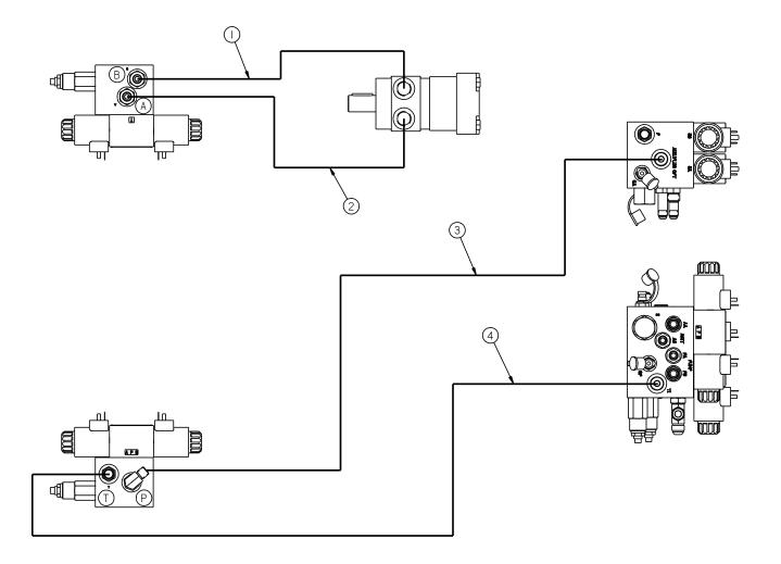
Figure 9.49 26605 Hydraulic Schematic EZ Series II 1500 Autoloade
