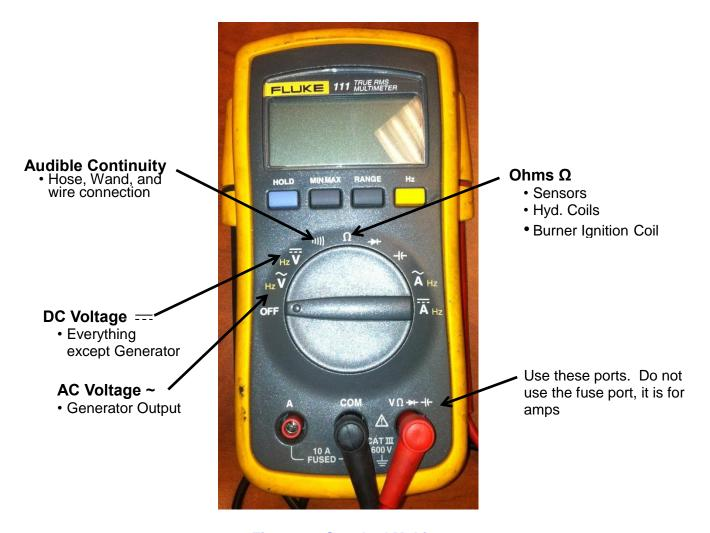
**Figure 7.1 Standard Multimeter**
