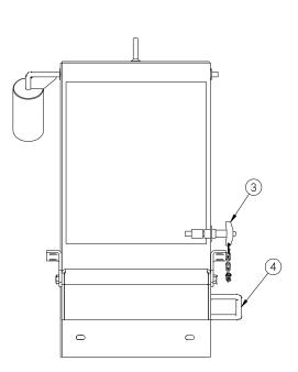
Figure 9.44 51375 Splash Box Welded Assembly LH
