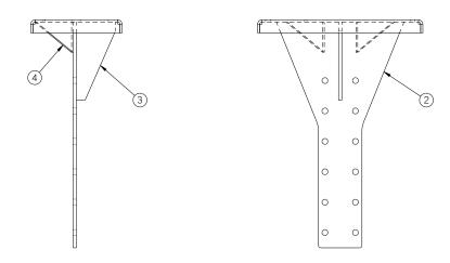
Figure 9.23 51253 Front Leg Support Mounting Plate Assembly
