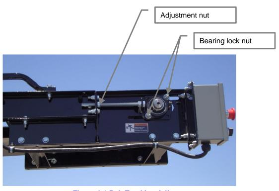
**Figure 6.1 Belt Tracking Adjustment**
