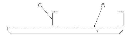
Figure 9.2 51302 Top Support-Cross Over Assembly
