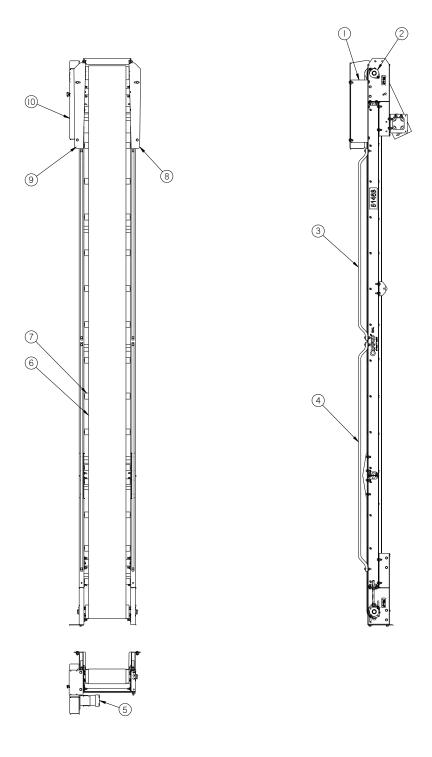
Figure 9.25 51430 13' Conveyor Assembly
