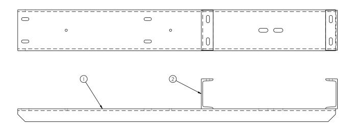
Figure 9.41 51392 Top Support-Cross Over Assembly
