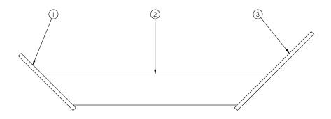
Figure 9.40 51255 Underbody Angled Support Brace
