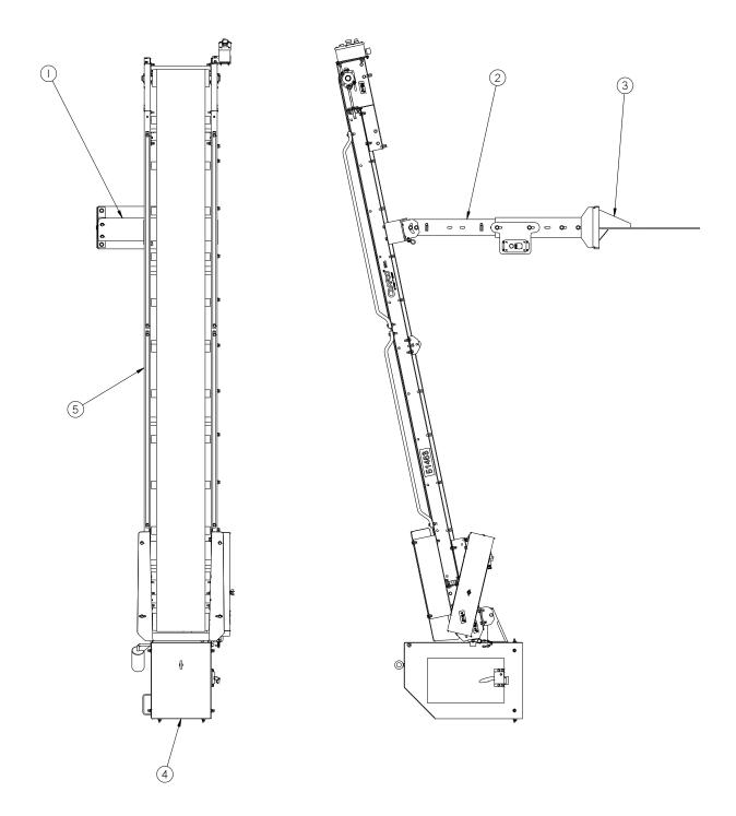
Figure 9.1 Super Shot 125 Diesel and Diesel Compressor Melter Autoloader Kit
