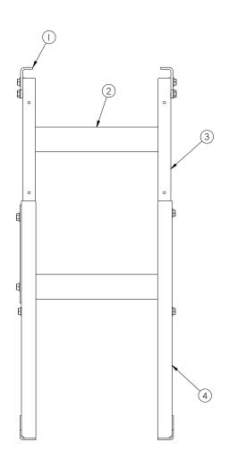
Figure 9.42 51113 Heavy Duty Structure Support
